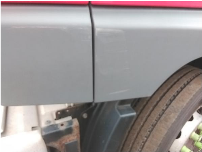
5: Qtr Panel Moulding os Scuffed (Unpainted) Over 100mm
