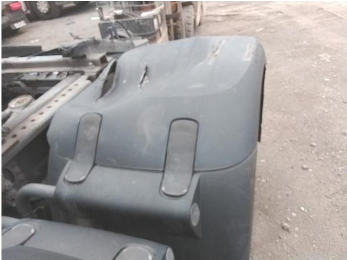
4: Qtr Panel Moulding ns Broken Replace
